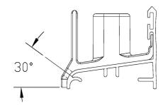
Step 30: Drill the 2 holes as marked, do not use a lot of pressure on the drill. If you need to check the location, use the Center Guide for the location and angle.
