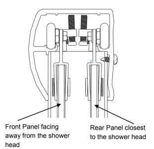
Step 26: The Inside Glass panel should be located by the Shower Head. Make sure you have good contact with the 3 bumpers. If not, remove the panel from the header and adjust the rollers to make good contact. MAKE SURE THAT THE ROLLER SCREWS ARE TIGHT Reinstall the panel as in Step 25
