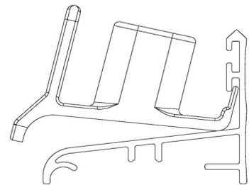
Step 29: Slide the Center Guide to either the Right or Left of the center of the Bottom Track. Measure and confirm that the Center Guide is in the middle. Mark the hole location with the Pencil. Move the Center Guide away from the marked locations. Using the Center Punch mark the hole centers at about a 30° angle. Use Caution not to move the bottom
